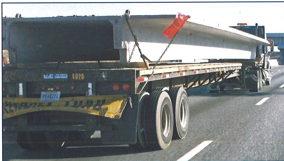
Figure 2 – Spans of 50 to 80 ft. are rather common, with some projects supplied in lengths in excess of this range. Transportation of precast tees may be the limiting factor in determining their maximum practical span.
