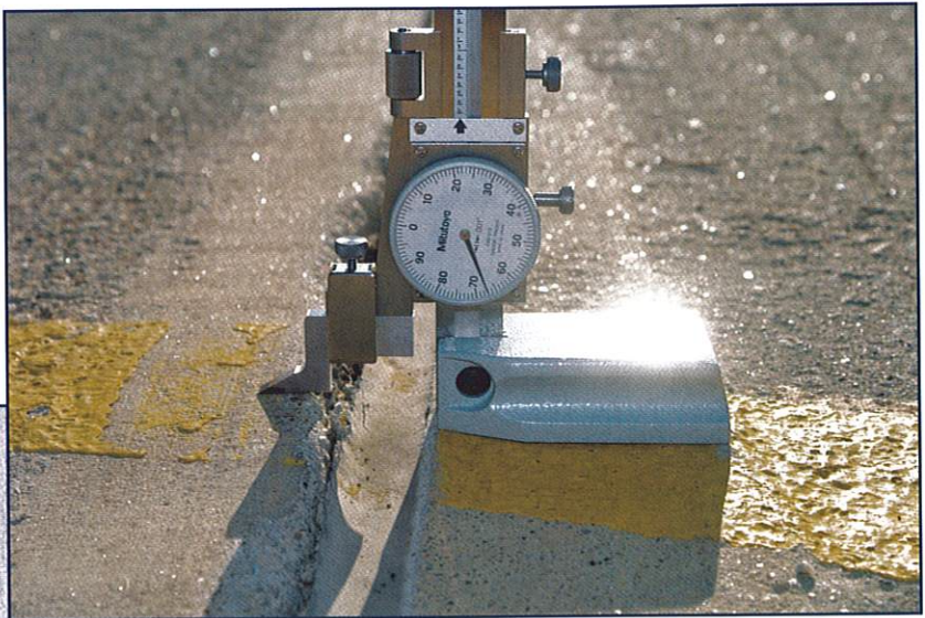
Figure 6 – Differential loading and stresses at connection brackets can result when adjacent panels are not the same height. Here, the difference in top-surface elevation is measured using a dial gauge micrometer.
