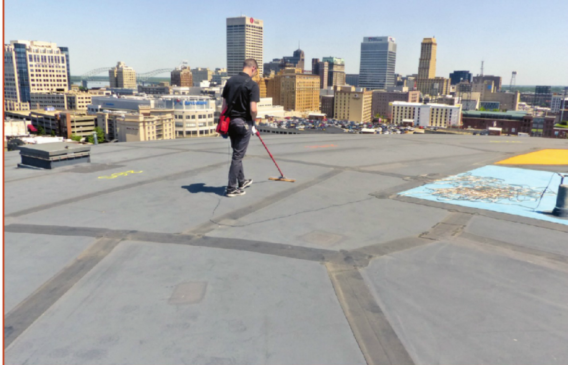
Figure 6. High-voltage electronic leak detection testing being performed.
