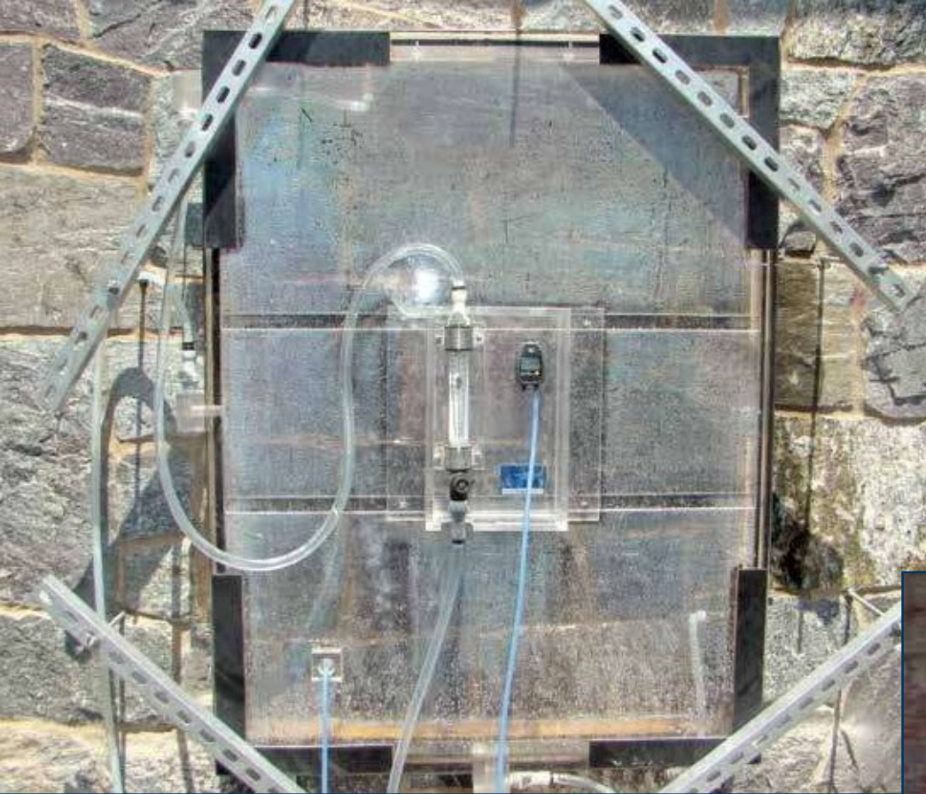
Photo 8 – Chamber securely anchored to masonry wall during an ASTM C1601 test.
