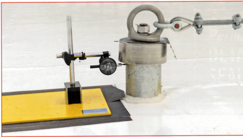
Figure 7 – Dial deflection gauge attached to adjustable stand and magnetic base fastened to a steel plate.
