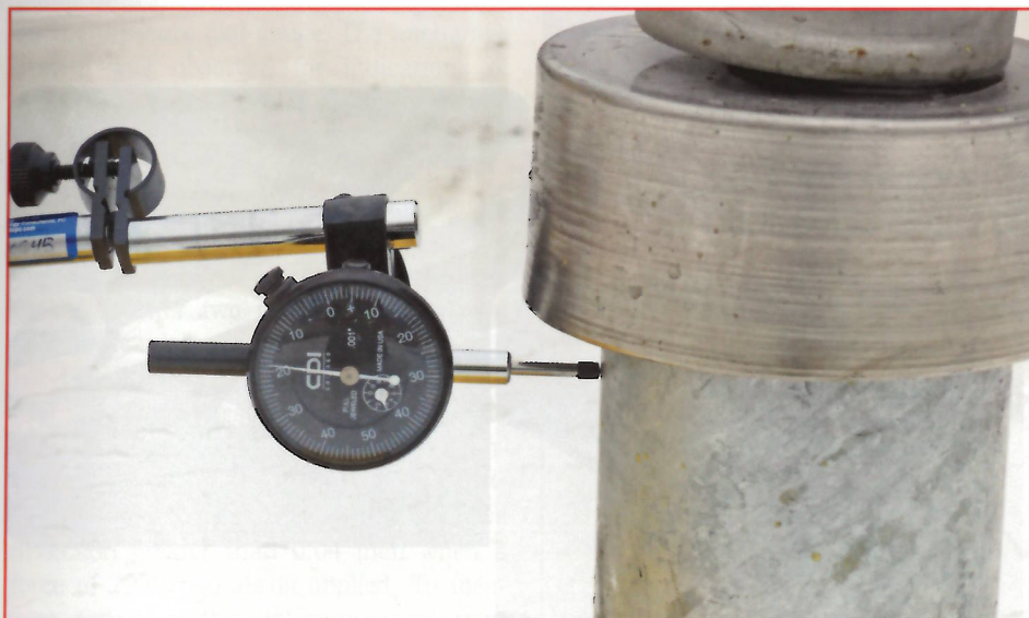
Figure 6 - Dial deflection gauge with gradations of 0.001 inch.
