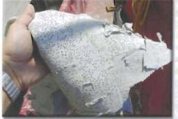
Extensive blistering within the TBM base coat due to excessive base coat thickness. 44 • INTERFACE
