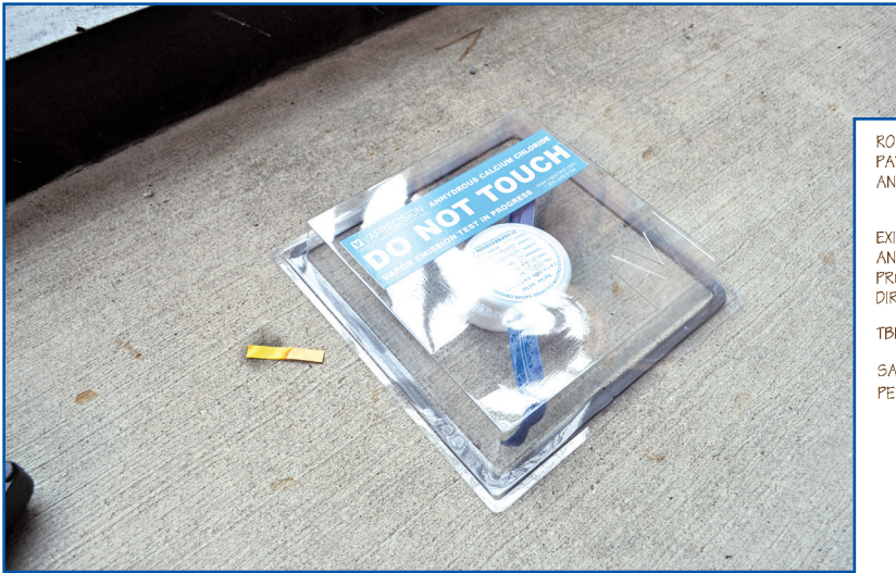
Figure 7 – ASTM F1869 moisture emission testing.
