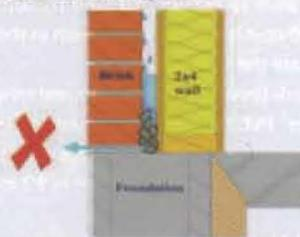
Water which is trapped between brick and wall can cause serious damage.
